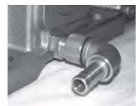
A brass drain valve is threaded into the existing oil drain port of the gearbox. The spring valve is closed using a rubber o-ring. When the hose fitting is threaded into the drain valve, the spring valve is pushed open and allows oil to drain. When the hose fitting is removed, the drain valve closes. A brass, threaded cap is supplied to cover the drain valve when not in use.
